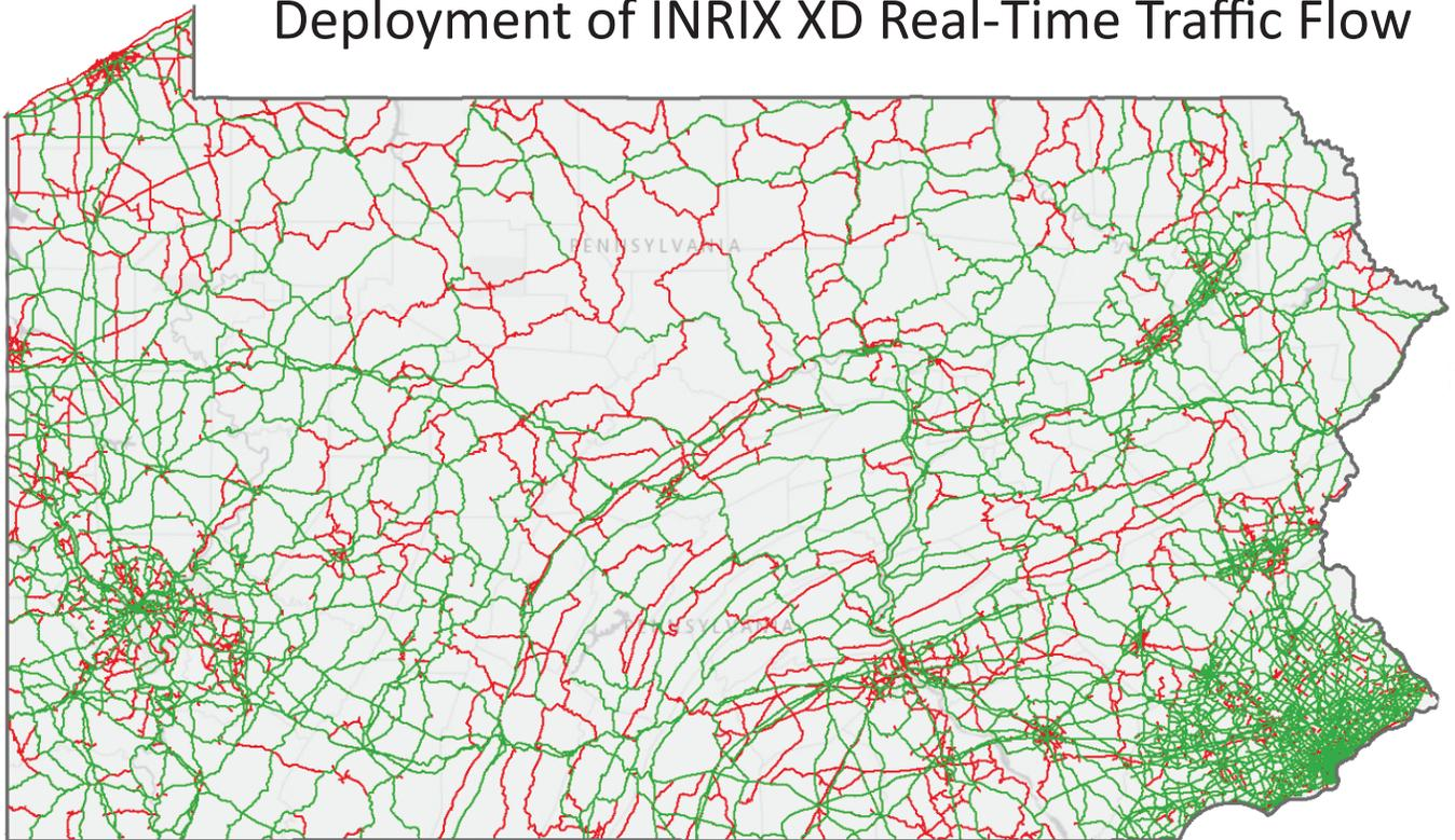
INRIX coverage in Pennsylvania. TMC coverage is shown in green while the additional XD coverage is shown in red. XD coverage adds over 15,000 centerline miles, a 50% increase over TMC coverage.
